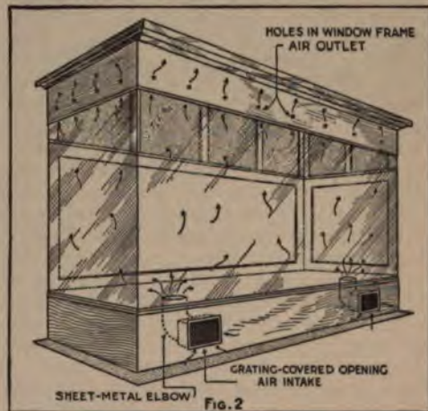
When the Lower Frame of the Window Does Not Extend above the Floor, Recourse must be Had to Two or Three Large Openings, Covered with Gratings
